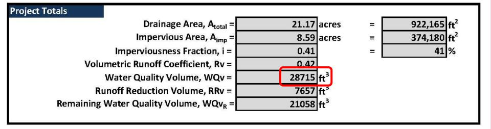
The difference in the calculations done previously and those by the spreadsheet is due to round-off error in the hand calculations.
